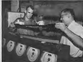
PRIOR TO a wind tunnel test, the above-water section of the model is being lowered into the section that would be below water when the tanker is carrying a full load. This is a "with cargo" test. PRIOR CU un prueba den un tanki di awa, e parti di e modelo cu ta keda ariba awa wordu hatai den un seccion cu ta keda baha awa ora e tanker ta completamente cargá. Esaki ta un prueba cu carga.
